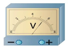
The units for potential difference is volts (or V)
