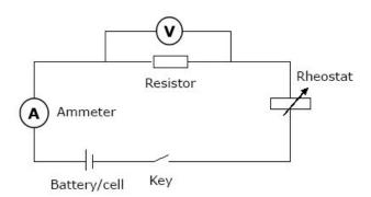
An ammeter must always be connected in a circuit in such a way that the current it measures flows directly through it. The ammeter is said to be connected in series in the circuit, in order
