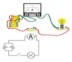
This includes the cell, the lamp, the switch and the wires connecting to the ammeter.
