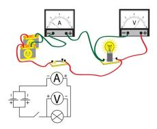
On the top right is the voltmeter, with the symbol V.
